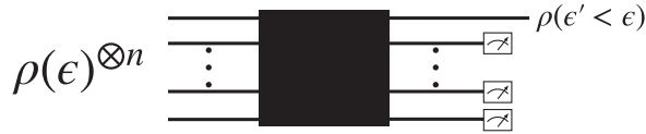
FIG. 1. Cartoon schematic of distillation scheme. n copies of a noisy photon state with error rate \epsilon [Eq. (3)], incident upon n spatial rails, are used to distill a single photon of lower error \epsilon' < \epsilon . This is achieved upon postselection of a particular detection pattern of n - 1 photons in the measured rails. The black box is at this point unspecified but will be an array of beam splitters between the rails to enact interference.
