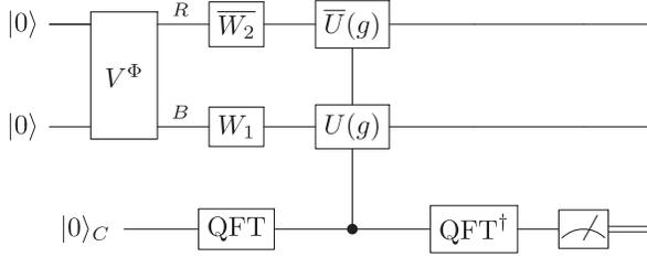
FIG. 1. Quantum circuit to test for the covariance of a unitary Hamiltonian evolution. The unitary  $V^\Phi$  generates the state  $|\Phi\rangle_{RA}$ , the maximally entangled state on  $RA$ . The evolution of the system is given by  $e^{-iHt} = W_1 W_2^\dagger$ , and the  $U(g)$  gates are controlled on a superposition over all of the elements  $g \in G$ , as in (4).
