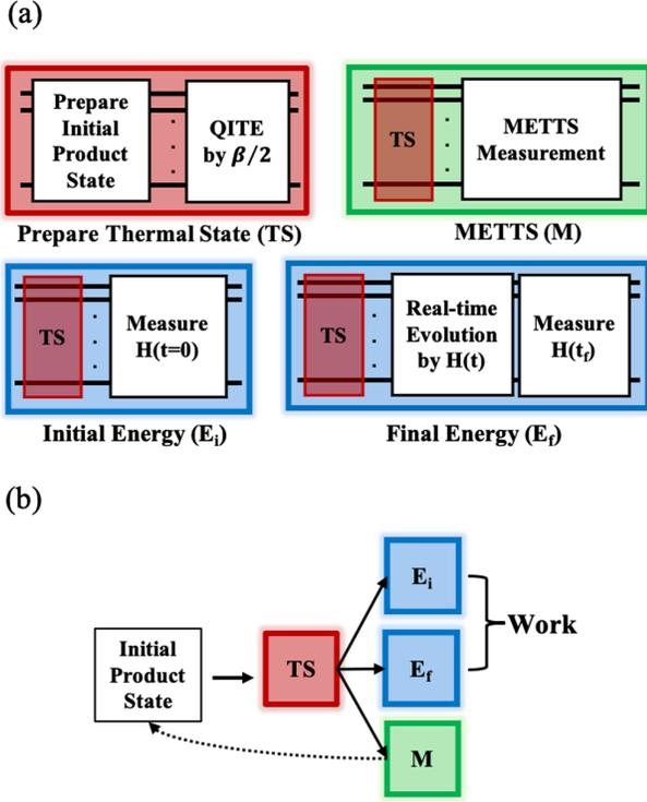
FIG. 2. Circuits generated and workflow diagram for the algorithm. (a) Quantum circuit diagrams for the thermal state preparation subcircuit (red), which is used in three separate circuits for measuring the initial and final energies (blue) as well as measuring the initial product state for the subsequent trajectory (green). (b) Workflow diagram depicting how the circuits above are integrated to produce a pseudowork distribution.
