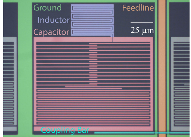
FIG. 1. A microscope image of a hafnium optical kinetic inductance detector coupled to a coplanar waveguide feedline. The image has been given false color to highlight the functions of each part of the device. The dark areas are the bare sapphire substrate. Light is focused onto the 47 \mu\text{m} \times 34.7 \mu\text{m} inductor with a microlens, which allows arrays of these detectors to achieve near unity fill factors. An approximate scale bar is included for reference.
