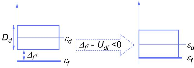
FIG. 4. Schematic of the promotional model in which valence transition is associated with the onsite charge transfer between  $4f$  and  $5d$  states, where  $U_{df}$  is the interorbital Coulomb repulsion between the carrier and localized hole on the same site,  $D_d$  is the bandwidth of  $5d$  band. Once the gap approaches  $U_{df}$ , the valence transition occurs.
