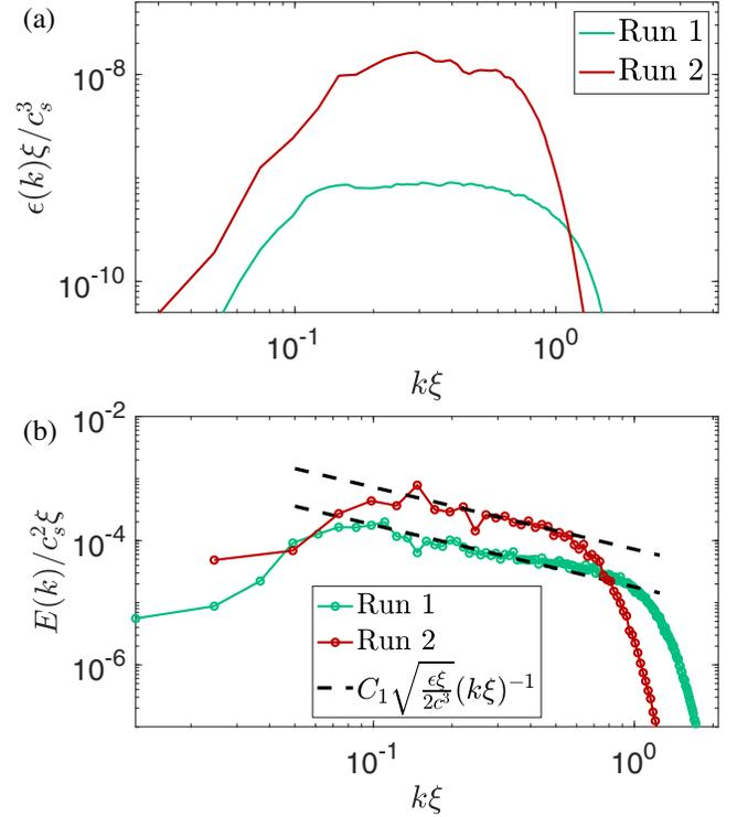
FIG. 2. (a) Energy flux. (b) Energy spectra. Dashed lines correspond to theoretical predictions (9) and (18) using the corresponding flux values in the inertial range.
