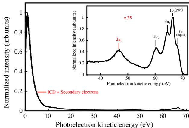
FIG. 2. Photoelectron spectrum of a liquid-water microjet recorded with XUV pulses centered at 79.0 eV (H51 of 800 nm).
