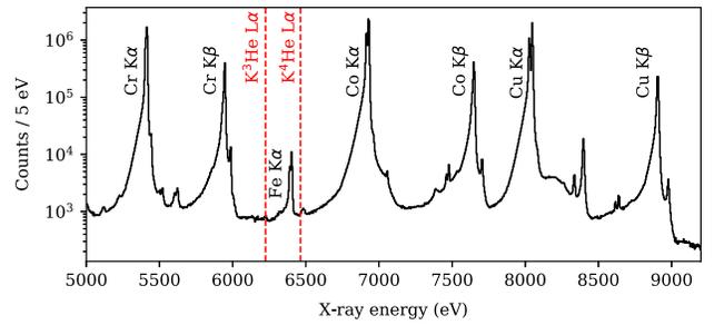
FIG. 1. TES-measured x-ray spectrum summed across all the  $^3\text{He}$  data. The characteristic lines used for the energy calibration are labeled. The expected  $3d \rightarrow 2p$  x-ray energies from the kaonic  $^3\text{He}$  and  $^4\text{He}$  are indicated as dotted lines. The small feature near 6500 eV, just above the  $K^{-4}\text{He}$   $L\alpha$  energy, is the Bi  $M\beta$  escape peak of the Cu  $K\beta$  line.
