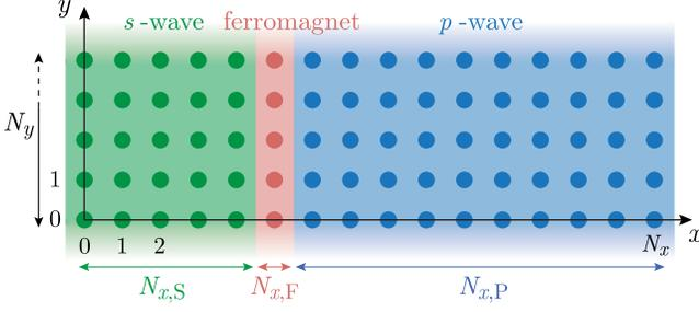
FIG. 1. Schematic illustration of the two-dimensional *SFP* cubic  $N_x \times N_y$  lattice structure, with layer thicknesses of  $N_{x,S}$ ,  $N_{x,F}$  and  $N_{x,P}$  lattice sites, respectively. The  $y$  direction is translationally invariant by using periodic boundary conditions and  $N_y \gg N_x$ .
