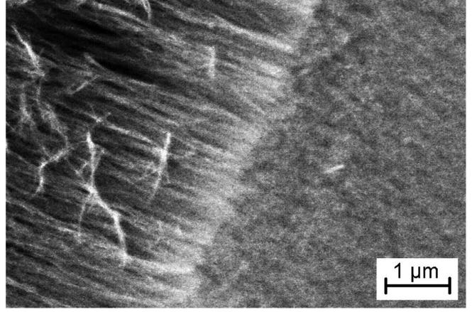
FIG. 1. Scanning electron microscope image of the free surface of mullite aerogel sample.
