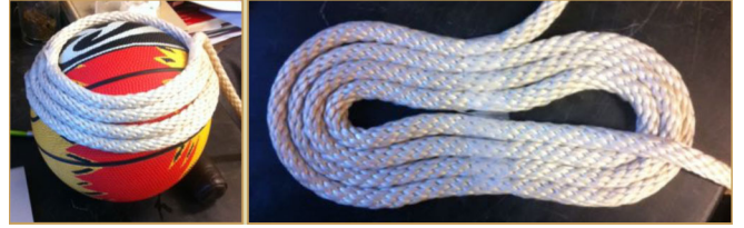
FIG. 5. A macroscopic demonstration of how the fiber coil can collapse to a flat surface, forming a unique, noncircular shape.
