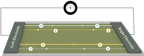
FIG. 2. Schematic of the experimental setup for measuring the nonlinear current. The voltages are measured along the left and right electrodes. Here the edge states occur in pairs having spin-up (blue) and spin-down (yellow). Thick lines refer to occupied states and thin lines to unoccupied states.
