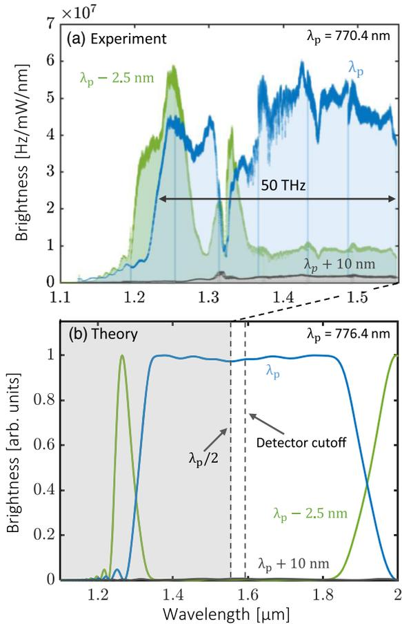
FIG. 3. (a) Signal spectrum at different pump wavelengths with  $\lambda_p$  corresponding to the pump wavelength that gives the widest spectrum. (b) The corresponding simulated plots for the designed waveguide.
