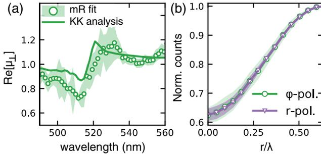
FIG. 4. (a)  $\text{Re}[\mu_{\perp}(\lambda)]$  derived directly from unconstrained MR analysis (markers) and from KK analysis (solid line) of  $\text{Im}[\mu_{\perp}]$ . Filled color region: standard deviation over all measurements. (b) Comparison of  $\text{BA}_2\text{PbI}_4$  PL under tightly focused (purple triangles)  $r$ -polarized and (green circles)  $\phi$ -polarized excitation.
