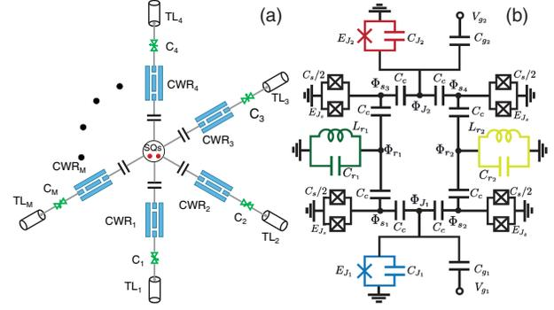
FIG. 3. (a) Schematic setup for the generation and release of the  $W$  state: Two SQs are capacitively coupled to  $M$  CWRs. Each CWR is connected to a TL through a variable coupler  $C$ , such that the photon emission rate into the TL is controllable. (b) A superconducting circuit design for the two-qubit two-mode Rabi model [56].
