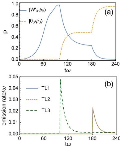
FIG. 5. Numerical simulation for the catch and release of the perfect three-mode  $W$  state  $|W'_3\rangle = \frac{1}{2}(|100\rangle + |010\rangle + \sqrt{2}|001\rangle)$  for quantum teleportation. (a) Population of different states inside resonators. (b) Emission rates into transmission lines.
