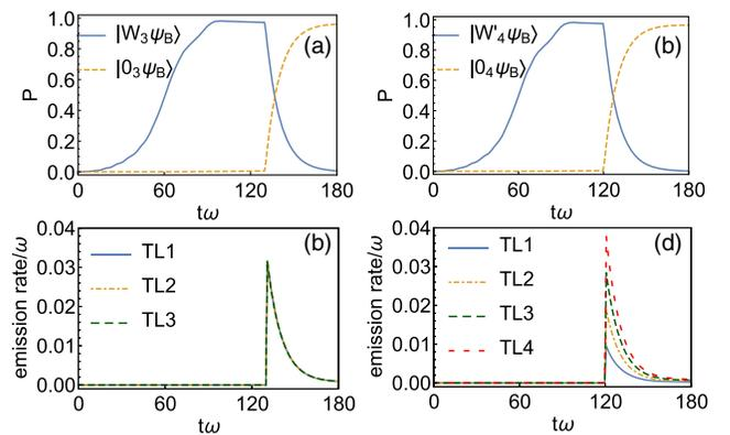
FIG. 4. Numerical simulation for the catch and release of the prototype three-mode  $W$  state  $|W_3\rangle = (1/\sqrt{3})(|100\rangle + |010\rangle + |001\rangle)$  (left panel) and the four-mode  $W$  state  $|W'_4\rangle = (1/\sqrt{10})(|1000\rangle + \sqrt{2}|0100\rangle + \sqrt{3}|0010\rangle + 2|0001\rangle)$  (right panel). (a) and (b) Population of different states inside resonators. (c) and (d) Emission rates into transmission lines.
