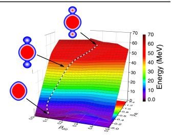
FIG. 3. Reflection symmetric deformation energy surface of  $^{224}$ Ra in the quadrupole-hexadecapole axially symmetric plane. Calculations are carried out using the RHB model based on the DD-PC1 functional, and separable pairing interaction. The black and white dashed curve denotes the dynamical (least-action) path for  $2\alpha$  emission from equilibrium deformation to scission, and the insets display the intrinsic nucleon densities for three selected points on the path.
