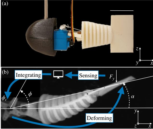
FIG. 2. (a) Side view of the fishlike robotic system: the white material is 3D printed using soft polymers. The tail is driven by two cables attached to a waterproof servomotor (blue piece). The swimmer is attached to a force sensor (vertical rod connected to the head). The thin white bar represents 3.5 cm. (b) Top view of the servomotor and the elastic tail.
