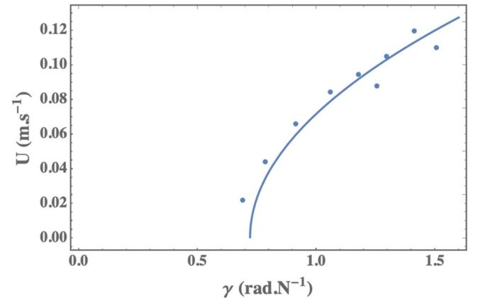
FIG. 5. Swimming velocity  $U$  as a function of the proprioceptive feedback parameter  $\gamma$ . The experimental points are shown as disks. The curve represents the fit  $U = 0.14\sqrt{\gamma - \gamma_c}$  in Systeme International units.
