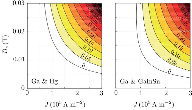
FIG. 2. Growth rate  $\lambda$  in  $\text{s}^{-1}$  of the fundamental wave ( $m = 1$ ,  $\kappa_{11} = 1.841$ ) in the  $J$ - $B_z$  plane in a  $R = H_1 = H_2 = 2$  cm setup with layers of Ga and Hg or Ga and GaInSn eutectic.
