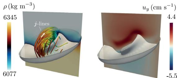
FIG. 6. Simulation with Ga and GaInSn eutectic (miscible setup) using exaggerated diffusion  $D_{\text{fake}} = 100D = 1.7 \times 10^{-7} \text{ m}^2 \text{ s}^{-1}$ ;  $J = 4 \times 10^5 \text{ A m}^{-2}$ ;  $t = 31.35 \text{ s}$ . The interface shown here is the isosurface  $\rho = (\rho_1 + \rho_2)/2$ .
