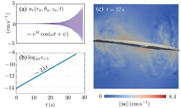
FIG. 4. Simulations in the immiscible Ga and Hg setup. (a) Time series of the velocity at  $r_a = 0$ ,  $\theta_a = 0$ ,  $z_a = -5$  mm gives  $\omega$ . (b) Time series of  $e_{c,1}$  gives  $\lambda$  ( $e_{c,1}$  is the kinetic energy of the azimuthal Fourier mode  $m = 1$ ). (c) Isosurface  $\rho = (\rho_1 + \rho_2) / 2$  and turbulent structures in the vertical plane  $x = 0$  at  $t = 37$  s.
