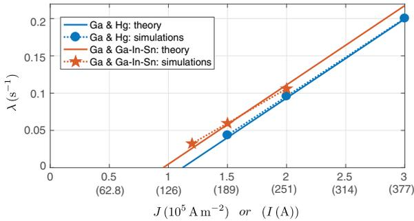
FIG. 3. Growth rate  $\lambda$  in  $\text{s}^{-1}$  of the fundamental wave ( $m = 1$ ,  $\kappa_{11} = 1.841$ ) as a function of  $J$  or  $I$  in a  $R = H_1 = H_2 = 2$  cm setup with magnetic field  $B_z = 15$  mT.
