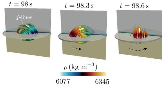
FIG. 5. Emergence of a rotating gravity wave in Ga and GaInSn eutectic (miscible) setup,  $J = 1.5 \times 10^5 \text{ A m}^{-2}$ . We show the isosurface  $\rho = (\rho_1 + \rho_2)/2$ , the density  $\rho$  in color code in the vertical plane  $x = 0$ , and lines of excess current  $\mathbf{j}$ .
