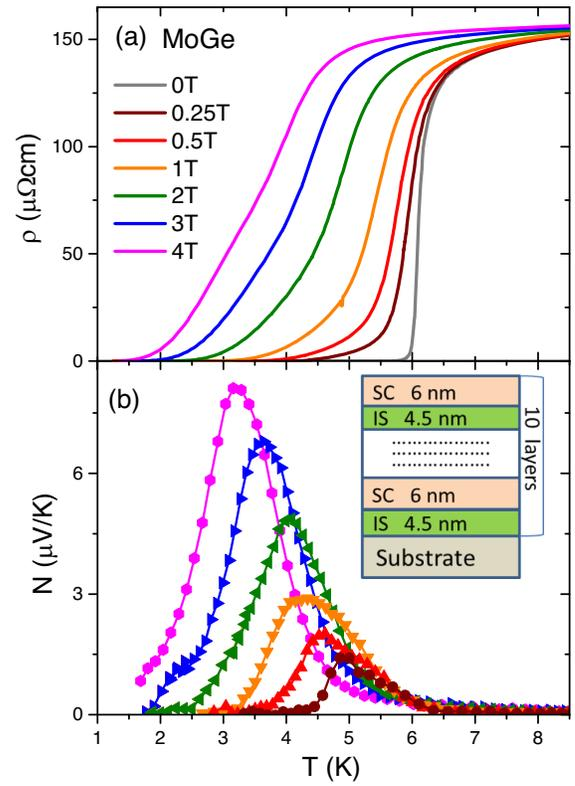
FIG. 3. Nernst effect in amorphous MoGe: (a) Evolution of the resistive superconducting transition in amorphous films of MoGe with magnetic field. (b) Nernst effect  $N$  in the same sample. The color code for magnetic fields is identical to the one used in the upper panel. The inset schematically depicts the structure of the sample consisting of alternating superconducting and insulating layers.
