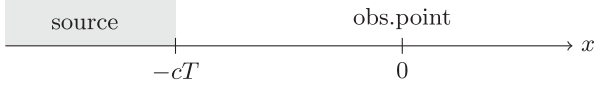
FIG. 1. A source is located in the region x < -cT , and we consider field observables at the observation point x = 0 . The source is turned on at t = -T , which means that the observables must be unchanged for t < 0 .
