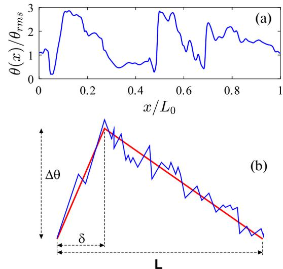
FIG. 1. (a) Typical one-dimensional trace of the scalar field in the direction of the imposed mean-gradient ( $x$ ), for  $R_\lambda = 140$  and  $Sc = 1$ , normalized by the rms value.  $L_0 = 2\pi$  is the domain length. (b) A cartoon of the ramp-cliff model, based on the trace (but not to scale).
