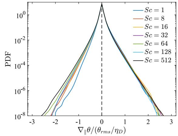
FIG. 7. PDFs of scalar derivative parallel to the imposed mean gradient, normalized by  $\theta_{\text{rms}}/\eta_D$ .  $R_\lambda = 140$ .
