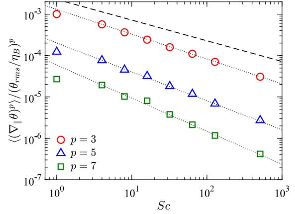
FIG. 4. The 3rd, 5th, and 7th order moments of the scalar derivative in the direction of the imposed mean gradient at  $R_{\lambda} = 140$ , suitably normalized by  $\theta_{\text{rms}}/\eta_B$ . Dashed line corresponds to the  $-1/2$ -power predicted by Eq. (3), whereas the dotted lines correspond to power laws with  $-1/2 - \alpha(p-1)$ ,  $\alpha = 0.05$  (see text). For clarity, the data for  $p = 5$  and  $7$  are shifted down by factors of 4 and 16, respectively.
