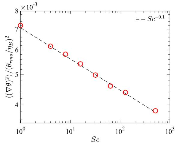
FIG. 5. The variance of scalar gradient (which is also given as  $\langle \chi \rangle / 6D$ ) normalized by  $\theta_{\text{rms}}/\eta_B$  at  $R_{\lambda} = 140$ . The data can be well represented by a power law of the form  $Sc^{-0.1}$ .
