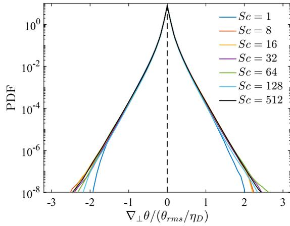
FIG. 6. The PDFs of scalar derivative in the direction perpendicular to the imposed mean gradient, normalized by  $\theta_{\text{rms}}/\eta_D$ .  $R_\lambda = 140$ . The statistical error bars are negligible and the probability density is shown here only when the number of samples in the histogram was greater than  $10^3$ . The exponential tails of these distributions was explored in Ref. [33].
