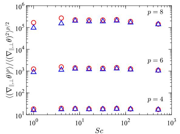
FIG. 8. Moments of scalar derivative in parallel (red circles) and perpendicular (blue triangles) directions of the imposed mean gradient. With increasing  $Sc$ , the moments approach each other and are also independent of  $Sc$ , affirming the collapses of the PDFs seen in Figs. 6 and 7.
