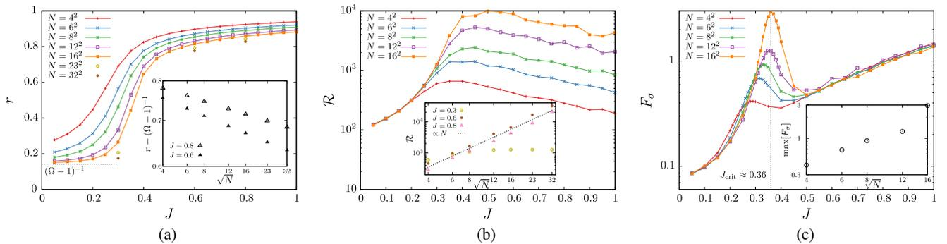
FIG. 3. Observables for the 2D variant as functions of the interaction strength  $J$ . (a) Order parameter  $r$ , which goes to zero in the thermodynamic limit for all  $J$ . (b) Number of coherent oscillations  $\mathcal{R}$  grows as power law. (c) Fano factor  $F_\sigma$  increases with system size.
