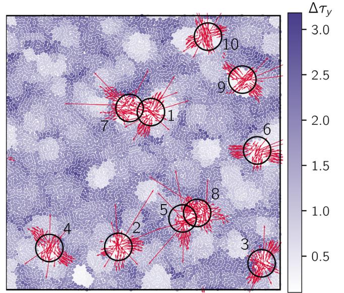
FIG. 4. Residual plastic strength map of a well-annealed Lennard-Jones binary glass at zero strain  $\gamma = 0$  (details about the model can be found in Ref. [59]). Black circles indicate the loci of the 10 first plastic instabilities. PHMs are extracted from the as-cast configurations by mapping the critical mode at each plastic event.
