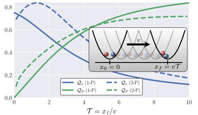
FIG. 1. Quality factors  $\mathcal{Q}_\nu$  and  $\mathcal{Q}_P$  for velocity and power, respectively, as a function of inverse driving speed  $\mathcal{T} = x_f/v$  for a moving trap. Solid lines (1-P): One particle,  $\beta = 10.0$ ,  $\mu = 1.0$ , and  $x_f = v\mathcal{T} = 10.0$ . Dashed lines (2-P): Two interacting particles as shown in the inset. The parameters are given in the Supplemental Material [62].
