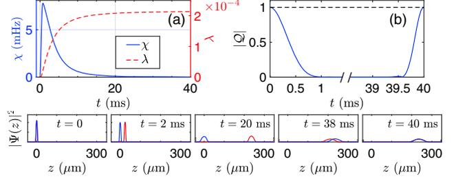
FIG. 2. Analytic spin squeezing model parameters determined from a GPE simulation of our scheme up to  $t = 2T_{\text{OAT}}$ , with  $T_{\text{OAT}} = 20$  ms and an  $N = 10^4$  atom BEC initially prepared in a spherical harmonic trap of frequency 50 Hz. (a) Effective squeezing rate  $\chi(t)$  (blue, solid) and squeezing degree  $\lambda(t)$  (orange, dashed). (b) Mode overlap  $|\mathcal{Q}(t)|$ . (Bottom) Normalized density slices at radial coordinate  $r = 0$ .
