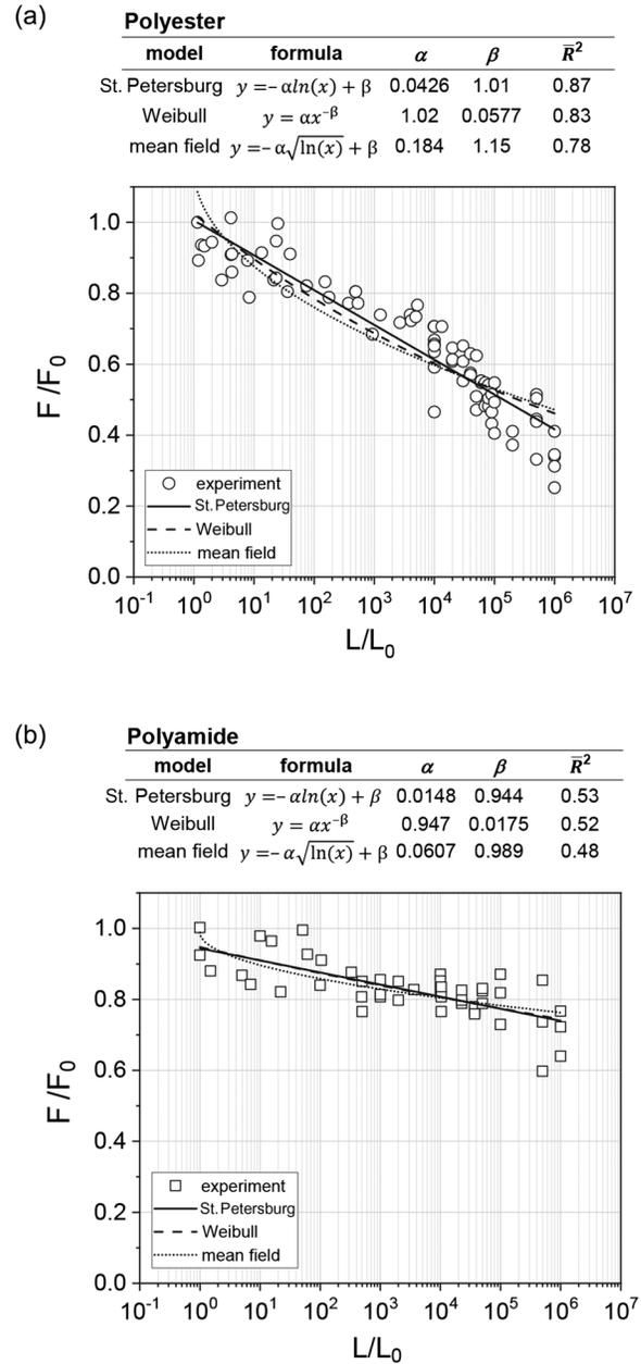
FIG. 2. Normalized fracture force for different length fibers. Normalized fracture force for the (a) polyester ( $L_0 = 1.2$  mm,  $F_0 = 17.84$  N) and (b) polyamide ( $L_0 = 1.0$  mm,  $F_0 = 42.60$  N) fibers as a function of fiber length from 1 mm to 1 km. The datasets were fit using the two parameter ( $\alpha, \beta$ ) St. Petersburg, Weibull, and mean-field models and are summarized in the tables above each graph.  $\bar{R}^2$  was used as a figure of merit.
