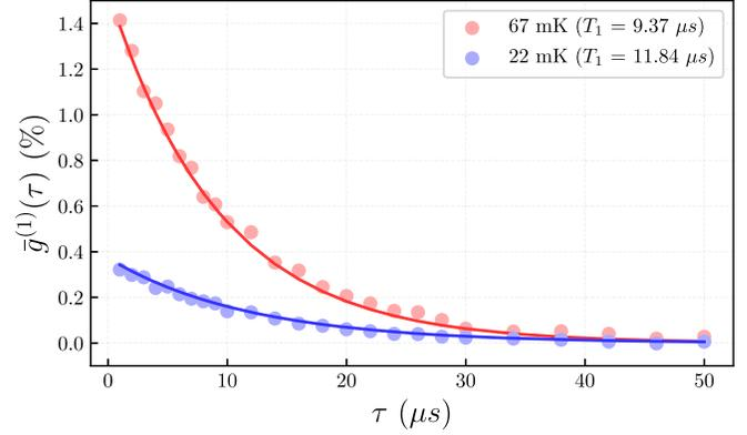
FIG. 1. Decay of the normalized correlator between two sequential measurements separated by  $\tau$ . The solid lines represent exponential  $T_1$  decay. Amplitude of the correlator at zero (or lowest attainable) delay allows one to reconstruct the  $|e\rangle$ -state population and hence the effective temperature of the qubit.
