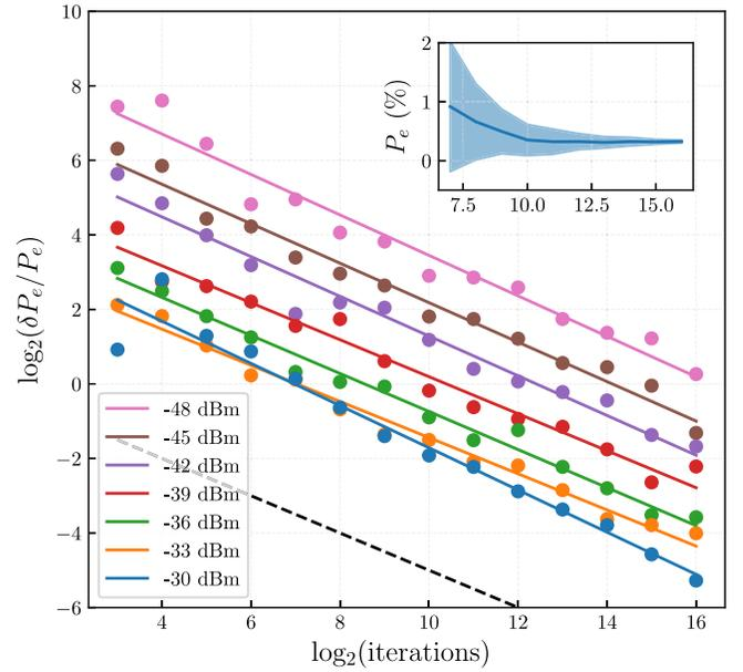
FIG. 5. Relative precision of  $P_e$  measurements and their linear fits. The precision scales as expected for uncorrelated noise (indicated by the black dashed line). Inset: Population (solid line) and standard deviation (fill) for a measurement power of  $-30$  dBm.
