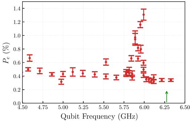
FIG. 4. Excited state population vs qubit frequency representing a “noise spectrum” as seen by the qubit. The green arrow indicates the qubit frequency used for the rest of the experiments.
