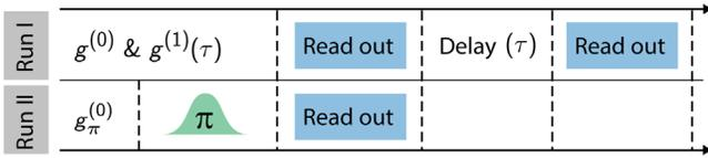
FIG. 2. The experimental protocol. “Run I” represents measurement of the correlation function  $g^{(1)}(\tau)$  and  $g^{(0)}$ . “Run II” is an additional calibration measurement required for correct scaling of  $P_e$ . The variable delay was used to measure the decay of  $g^{(1)}(\tau)$ . To determine  $P_e$  only one measurement with  $\tau = 0$  is necessary.
