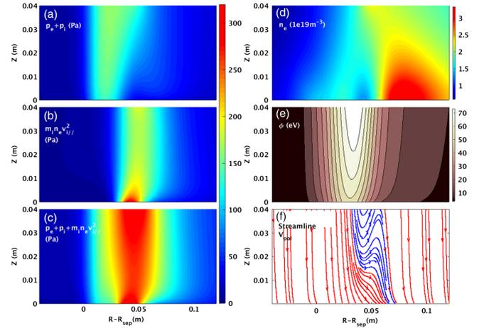
FIG. 3. Modeling results of 2D contour plot of (a) static ion and electron pressure, (b) ion dynamic pressure, (c) total pressure, (d) density, (e) plasma potential and (f) streamline of total poloidal flow. The blue lines show the stagnation of total poloidal flow at upstream.
