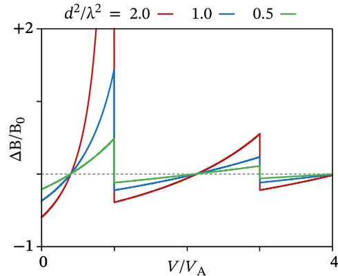
FIG. 3. Magnetic shift in the normal metal as a function of the applied voltage. Different curves correspond to different thicknesses  $d$  of the normal metal. Note that when  $d > \lambda$ , the paramagnetic effect produces a field  $B_0 + \Delta B$  many times larger than the applied field  $B_0$ .
