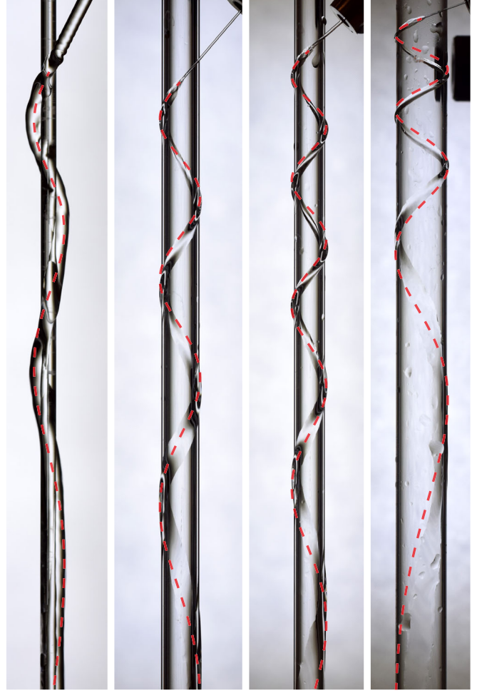
FIG. 3. Comparison between experiments and theory for a range of experimental parameters. From left to right: D_c = 1, 5, 10 mm; D_j = 1, 0.3, 0.5, 0.3 mm; \psi_0 = 26.3, 40.3, 47.8, 68.6 deg; U_0 = 1.0, 4.9, 3.0, 5.4 m/s; C = 15, 11.5, 7, 9.5 .
