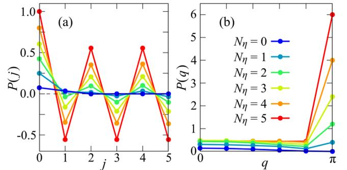
FIG. 3. (a) On-site pair-correlation function  $P(j)$  and (b) structure factor  $P(q)$  for  $|\psi_{N_\eta}\rangle$  at  $U = 8t_h$  with the different number of  $\eta$  pairs  $N_\eta (\leq L/2)$ .  $|\psi_{N_\eta}\rangle$  is generated from the ground state  $|\psi_{N_0, N_0}^{(\text{GS})}\rangle$  of  $\hat{\mathcal{H}}$  with  $N_0 = L/2 - N_\eta$  calculated by the ED for  $L = 10$  under PBC.
