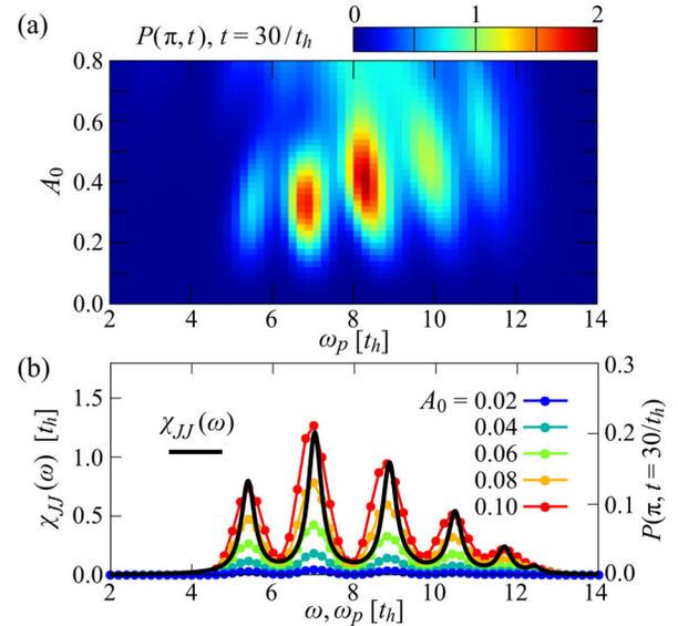
FIG. 2. (a) Contour plot of the pair structure factor  $P(q = \pi, t)$  at  $t = 30/t_h$  with varying  $\omega_p$  and  $A_0$ . (b) The GS optical spectrum  $\chi_{JJ}(\omega)$  is compared with  $P(q = \pi, t = 30/t_h)$  as a function of  $\omega_p$  for different values of  $A_0$ . The results are calculated by the ED method for  $L = 14$  at  $U = 8t_h$ , with  $\sigma_p = 2/t_h$  and  $t_0 = 10/t_h$ .
