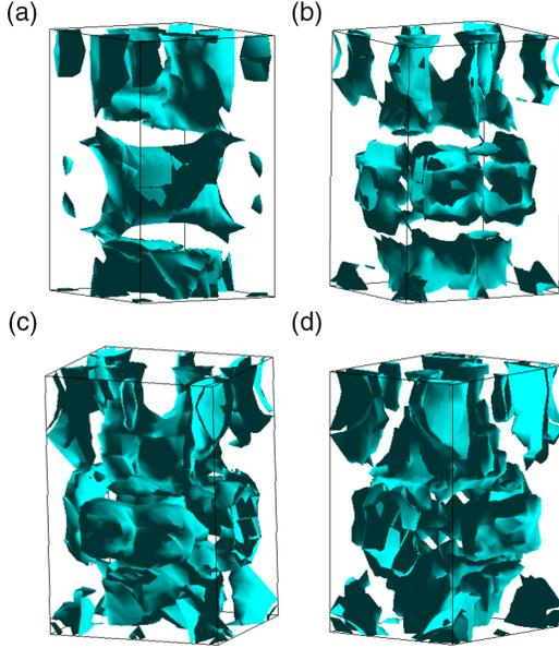
FIG. 2. The Fermi surfaces of Eu at the relative volumes (with respect to that at 75 GPa) of +6%, 0, -4%, and -10%. At all volumes the surfaces are large and multisheeted, varying through changes in topology with the only effect being the decrease in exchange constants and hence the ordering temperature, which vanishes around 82 GPa.
