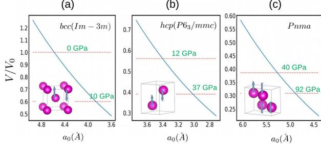
FIG. 1. The relative volume  $V/V_0$  ratio as a function of the  $a$  lattice constant (a) bcc, (b) hcp, and (c)  $Pnma$ . The lattice structures were obtained from experiments. Red dashed lines indicate the  $V/V_0$  ratio of pressures where the structures are confirmed stable in experiments, as given by Bi *et al.* [5].
