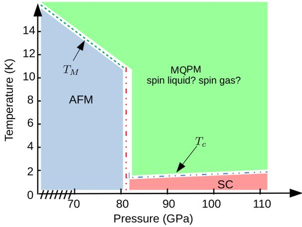
FIG. 4. Schematic depiction of the experimental phase diagram of Eu under pressure, showing the first order transition at  $P_c = 82$  GPa. Phases are these: MQPM, metallic quantum paramagnetic; AFM, antiferromagnetic; SC, superconducting.
