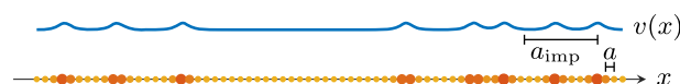
FIG. 1. Illustration of a velocity v(x) effectively describing a lattice system with impurities varying on a mesoscopic scale a_{\text{imp}} much larger than the lattice spacing a . For the XXZ spin chain described in the main text, x = ia , and the color and size of the dots indicate the magnitude of the couplings J_i .
