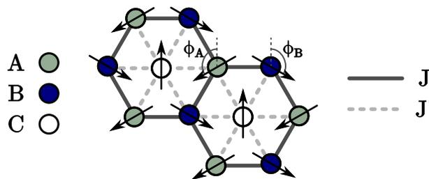
FIG. 1.  $\sqrt{3} \times \sqrt{3}$ -distorted triangular lattice, with two different exchange interactions  $J$  and  $J'$ . The arrows correspond to the spin directions of the semiclassical magnetic order.
