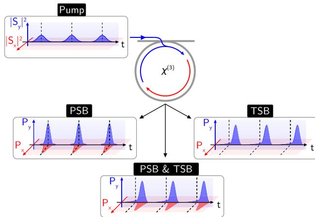
FIG. 1. Schematic of the different types of symmetry breaking in a dielectric ring resonator. By convention, the pump field is linearly polarized along the  $y$  axis. PSB: polarization symmetry breaking, TSB: temporal symmetry breaking.
