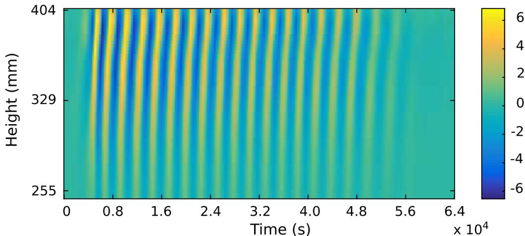
FIG. 2. Space-time diagram of the mean flow. The color code indicates the velocity in  $\text{mm s}^{-1}$ .  $N = 2.16$  Hz ( $\text{MgCl}_2$ ) and  $T_f = 15$  s.  $M$  changes every 8000 s:  $M = 14.5, 14, 13.5, 13, 12.5, 12, 11.5, 10.5, 10$  mm.
