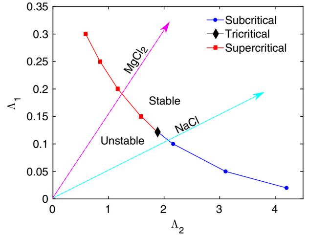
FIG. 5. Parameter space displaying the transition between stable (no mean flow) and unstable regions. Instability threshold for large  $N$  ( $\text{MgCl}_2$ ) and small  $N$  ( $\text{NaCl}$ ). Supercritical (filled square), subcritical (filled circle), and tricritical (filled diamond) transitions.
