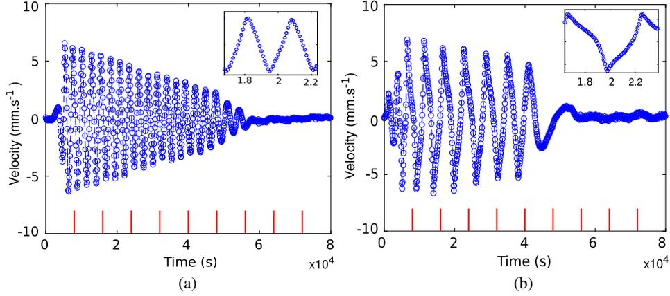
FIG. 3. Mean flow as a function of time, for two different values of  $N$ , at height  $h = 376$  mm.  $M$  changes every 8000 s (shown by vertical lines):  $M = 14.5, 14, 13.5, 13, 12.5, 12, 11.5, 10.5, 10$  mm. (Insets) details. (a)  $N = 2.16$  Hz ( $\text{MgCl}_2$ ). (b)  $N = 1.55$  Hz ( $\text{NaCl}$ ).
