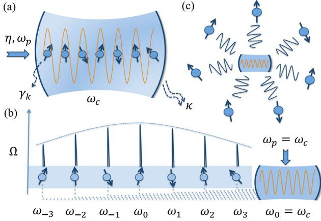
FIG. 1. (a) A mesoscopic spin ensemble interacting with a cavity, resonant at frequency  $\omega_c$ . The cavity is driven by a coherent pulse of strength  $\eta$  and frequency  $\omega_p$ . The cavity and spin losses are given by  $\kappa$  and  $\gamma_k$ . (b) The spin transition frequencies  $\omega_j$  in the ensemble form a spectral frequency comb, with collective coupling strength  $\Omega$ . (c) The spin-cavity system can be considered as a central body system.
