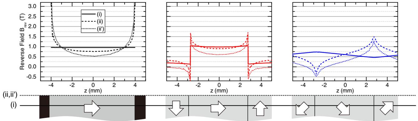
FIG. 5. Profiles of  $B_{\text{rev}}$  inside the REPM blocks of (a) the hybrid, (b) normal Halbach, and (c) 45° Halbach arrays, calculated along  $z$  at the vertical positions (i) 6 mm below the surface, and (ii), (ii') on the surface of each array. The cross sections of REPM blocks are shown at the bottom with the magnetization vectors.
