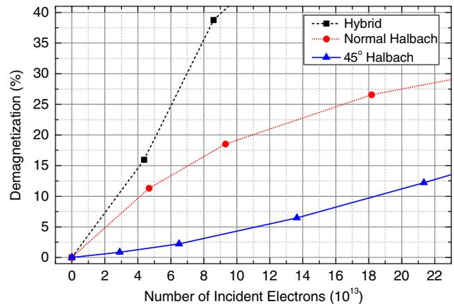
FIG. 4. Demagnetization of each undulator sample evaluated as the variation of the peak magnetic field, plotted as a function of the number of incident electrons.
