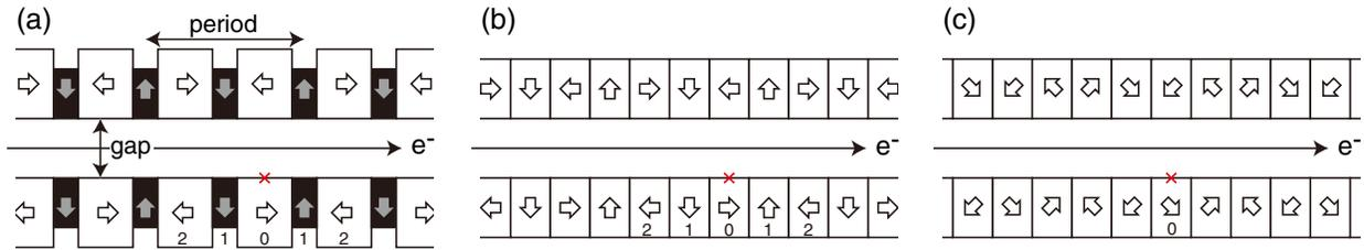
FIG. 1. Cross sections of magnetic arrays: (a) hybrid, (b) normal Halbach, (c)  $45^\circ$  Halbach undulators.
