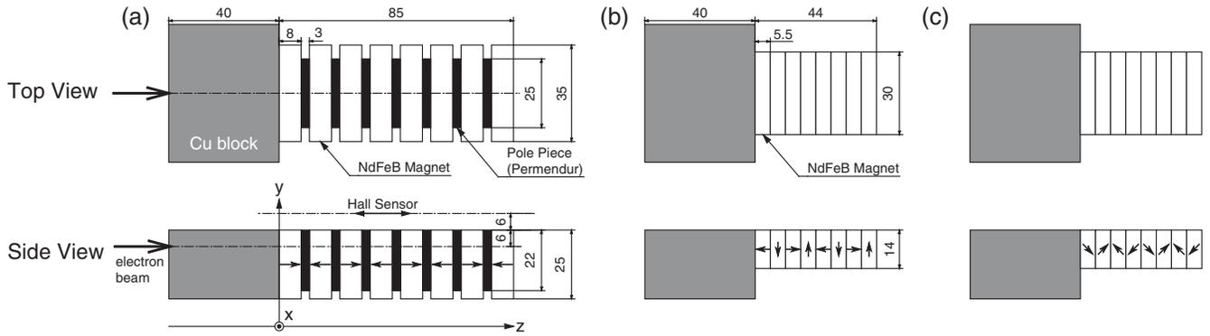
FIG. 2. Structures and dimensions of the undulator samples used for the irradiation experiments, consisting of the (a) hybrid, (b) normal Halbach, and (c)  $45^\circ$  Halbach arrays. The top and bottom figures correspond to the top and side views.
