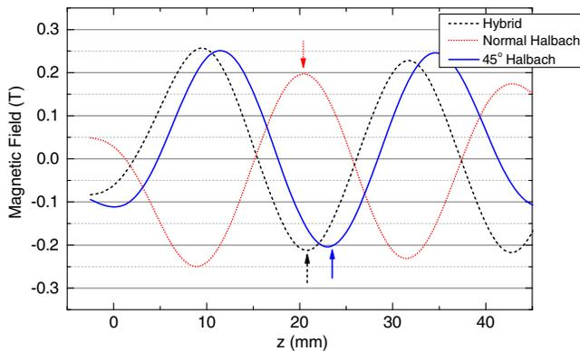
FIG. 3. Magnetic distributions of the three magnetic arrays measured by a Hall sensor along  $z$  before irradiation. Arrows indicate the peak positions to evaluate the demagnetization for respective magnetic arrays.
