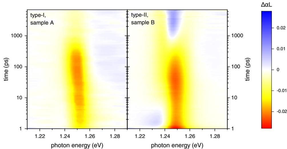
FIG. 2. Left panel: Contour plot of the optical pump-optical probe spectra for the reference sample *A* with a type-I band alignment. Right panel: Contour plot for sample *B* with a type-II band alignment and a 1.5 nm thick GaAs barrier. The plot illustrates the changes of the absorption ( $\Delta\alpha L$ ) after an optical excitation for time delays ranging from femtoseconds to several nanoseconds. In order to plot a logarithmic time scale the optical excitation is set to 1 ps.
