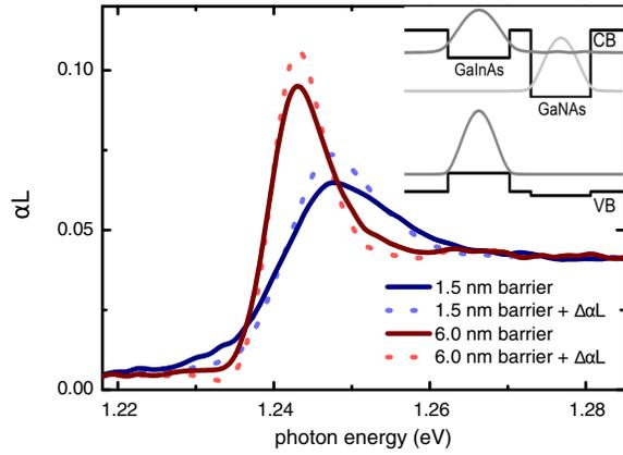
FIG. 1. Solid lines: Linear absorption spectra of the QW samples with a type-II band alignment and 1.5 nm (blue, sample *B*) and 6.0 nm (red, sample *C*) thick barriers, respectively. Dashed lines: Sum of the linear absorption and its respective differential absorption for a pump-probe delay of 5 ns. The inset is a schematic of the band diagram together with the corresponding wave functions.
