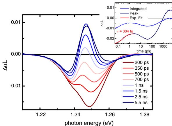
FIG. 3. Differential absorption spectra of sample *B* for different time delays. The inset shows transients at 1.248 eV (peak) as well as integrated over the whole bleaching signature from 1.215 to 1.28 eV (integrated).
