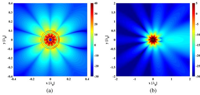
FIG. 5. Plots of  $10 \log_{10} |H_z(x, y)|$  for the MLS-excited, five-layer highly subwavelength cylinder. (a) Near field (the red dot denotes the source location). (b) Far field (the white dot denotes the source location).
