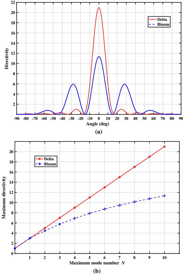
FIG. 3. Directivity obtained for the Dirac-delta- and binomial-distribution-based scattered field coefficients. (a) Patterns for  $N = 10$ . (b) Maximum directivity as the maximum mode number  $N$  varies (linear scales).
