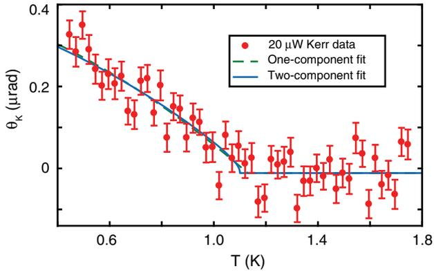
FIG. 3. Averaged Kerr data taken on sample E at  $20 \mu\text{W}$  incident power. Error bars are statistical errors (one- $\sigma$ ). Fits with two critical temperatures (solid blue line) or one (dashed green line) are overlaid.
