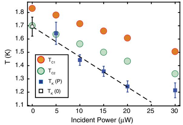
FIG. 4. Measured values of  $T_{C1}$  (orange circles),  $T_{C2}$  (light green circles), and  $T_K$  (blue squares) as a function of optical power on sample C. Error bars indicate 95% confidence intervals on the values of  $T_K$  extracted from Kerr data fits. The dashed line is a linear fit to  $T_K(P)$  from 5–20  $\mu\text{W}$ , extrapolating to  $T_K(0) = 1.694 \pm 0.072$  K (white square), which is consistent with  $T_{C2}$ .
