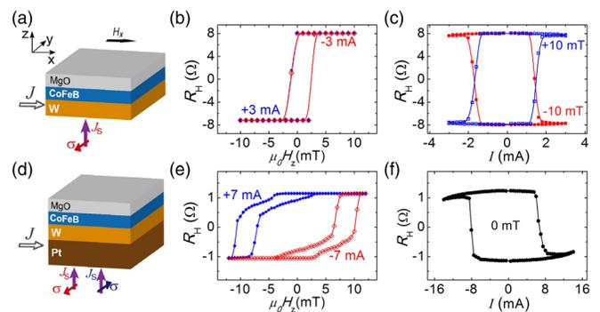
FIG. 1. Structures and current-induced switching behaviors in CoFeB with PMA, patterned with  $\alpha = 0^\circ$ . (a) Conventional SOT switching in W(1)/CoFeB(1)/MgO(1.8), (b) anomalous Hall effect (AHE) effect under +3 mA (blue solid circles) and -3 mA (open diamond circles), and (c) switching requiring a magnetic field. (d) Competing SOT effects of Pt/W/CoFeB/MgO. (e) AHE under positive and negative current. (f) Current induced magnetization switching requiring no magnetic field.
