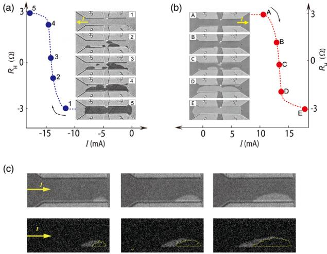
FIG. 3. MOKE images of current switching in Hall bar of Pt(2.5)/W(1.0)/CoFeB(1) for (a) increasing  $-I$  in the order of 1, 2, 3, ... and (b) increasing  $+I$  in the order of A, B, C, ... (c) Images after successive current pulses asymmetrically enlarging the domains at one end. In the lower panel, the yellow boundaries show the domains just before the current pulse, illustrating the contribution of the one current pulse.
