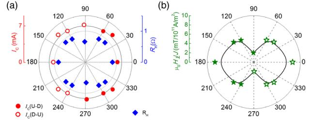
FIG. 4. Anisotropy of ZFS in Pt(3)/W(1.1)/CoFeB(1)/MgO(2) (in nm). (a) Angular dependence of the  $R_H$  values,  $I_C$ , and (b)  $\mu_0 \mathbf{H}_\perp / J$  values, where the solid and open circles indicate magnetization switching from up to down and down to up, respectively.
