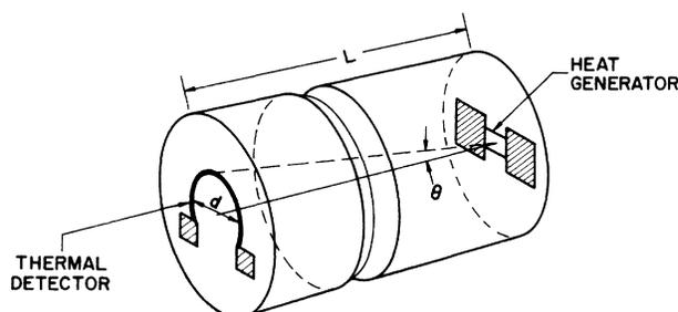
FIG. 1. Schematic diagram of the sample (length  $L$ ) showing the circular detector (diameter  $d$ ), the square heat pulse generator, and the peripheral cut made to control the scattered phonons. The annular detector width is 0.004 in. The shaded areas are evaporated silver "lands." The phonon trajectories lie along and near the cone of angle  $\theta$ .
