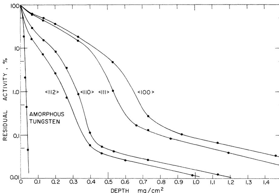
FIG. 1. Integral penetration distributions for 40-keV <sup>125</sup>Xe in tungsten. (Note that 1 mg/cm<sup>2</sup> is equivalent to 0.52 micron.)
