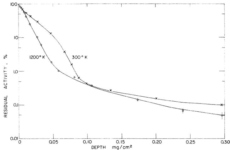
FIG. 4. Effect of lattice temperature on the penetration of 5.0-keV  $^{133}\text{Xe}$  along the  $\langle 100 \rangle$  direction.
