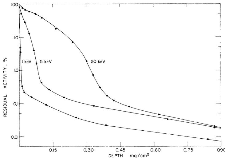
FIG. 3. Integral penetration distributions for  $^{133}\text{Xe}$  along the  $\langle 100 \rangle$  direction at various incident energies. (1  $\text{mg/cm}^2$  is equivalent to 0.52 micron.)
