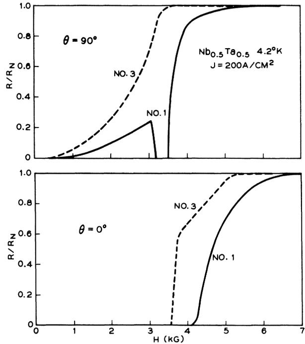
FIG. 3. Resistive transitions observed in Nb-Ta sheets. Sheet No. 3 is the same sample as shown in Fig. 1. Sheet No. 1 is identical to No. 3, but no annealing was applied to this sample.
