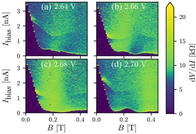
FIG. 2. (a)–(d)  $dV/dI$  vs  $B$  and  $I_{\text{bias}}$  for different gate voltage settings  $V_g$  indicated above each panel. Data from device 2; see the Supplemental Material [25] for the scanning electron micrograph of the device with the tuned gate marked.
