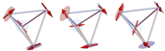
FIG. 1. Sketch (on a single tetrahedron) of three Palmer-Chalker configurations forming distinct magnetic domains below T_N (three others are obtained by reversing all spins). The local XY planes perpendicular to the \langle 111 \rangle axes are indicated by colored disks. Spins are pairwise antiparallel, and collinear with an edge of the tetrahedron. These configurations can be described as chiral spin crosses.
