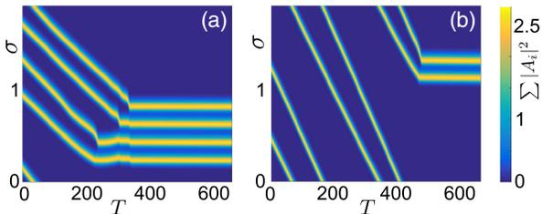
FIG. 3. (a) Space-time diagram of the bound pulse train regime in a four-laser array in coordinates  $(T, \sigma)$ , where  $\sigma = t \bmod \tau_0$  is the original fast time and  $T = t/\tau_0$  the slow time ( $\tau_0 = 1.9054$ ). Brighter colors indicate higher values of the sum of the laser intensities  $\sum_{i=1}^4 |A_i|^2$ . (b) Space-time diagram for the pulse train bound state regime for two lasers ( $\tau_0 = 1.9043$ ). Coupling parameters are  $\eta = 0.5$  and  $\varphi = 3.0$ .
