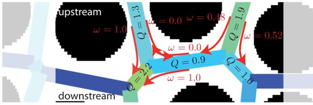
FIG. 2. Example of normalized flows  $Q/\text{mean}(Q)$  (black) and fractions of propagated flows  $\omega$  (red). At a node point, flows from incoming tubes slit up in fractions, for example  $\omega = \{1.0, 0.0\}$  or  $\omega = \{0.47, 0.52\}$ , top left and right, respectively. Kirchhoff's law ensures that fractions sum up to one. Flow in a tube downstream sums up flow contributions from tubes upstream, for example  $2.2 = 1 \times 1.3 + 1 \times 0.9$ , bottom left.
