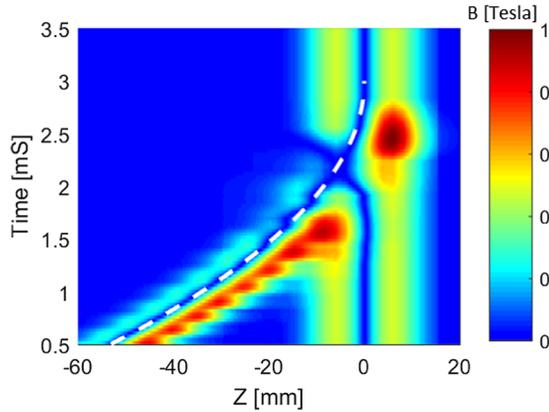
FIG. 2. Loading sequence of the static magnetic trap, showing the magnetic field magnitude along the  $Z$  axis as a function of time. Additional coils are used to cancel the front permanent magnet's field at the right time to allow the molecules to enter the static trap. The minimum of the magnetic field closely follows a trajectory of constant deceleration (dashed white line) that reaches zero velocity at the static trap's center.
